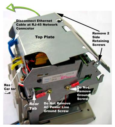
Figure 2-4. Top Plate Removal.
